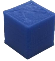
Figure 7: 3D-Printed Test Specimen for Density Measurement
