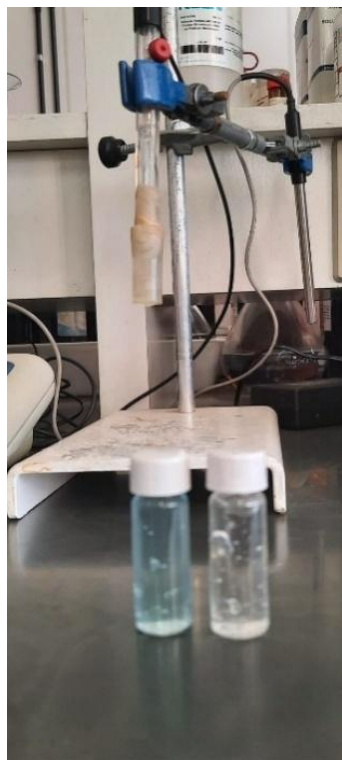
Figure 1: Samples of PPA gel/ \text{CuSO}_4 \cdot 5\text{H}_2\text{O} (bluish) and PPA gel (colorless) and separated in a vial for the irradiation process.
