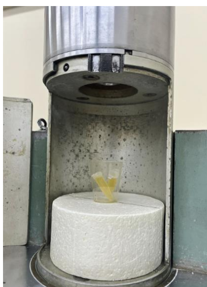
Figure 3: Samples in the Co-60 irradiator - GammaCell 220.
