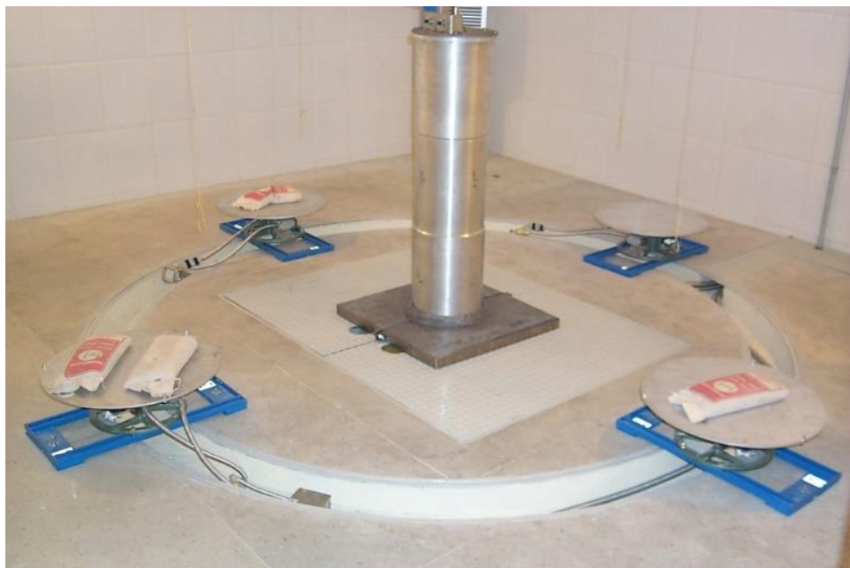
Figure 2: Cobalt-60 supply position and turntables.
