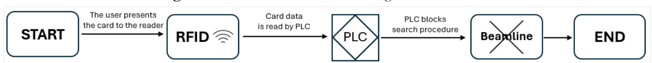
Figure 8: Data flow for PLC blocking forbidden cards
