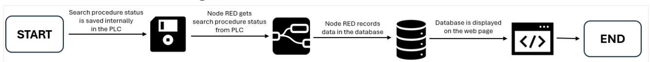
Figure 6: Data flow from PLC to the database
