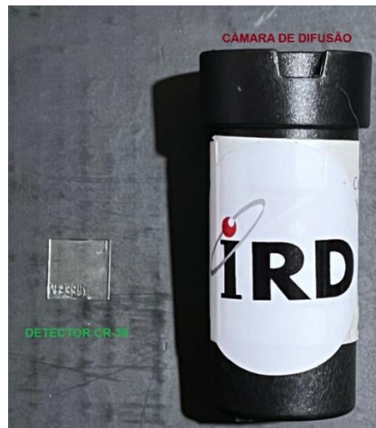
Figure 1: Diffusion chamber Radosys and CR-39 SSNDT detectors.
