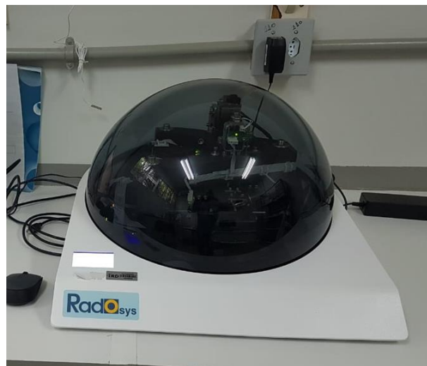
Figure 4: Radometer equipment for counting traces in CR-39 detectors.
