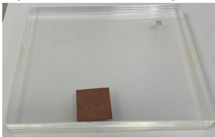
Figure 3: Standard phantom/simulator manufactured according to the IAEA methodology.
