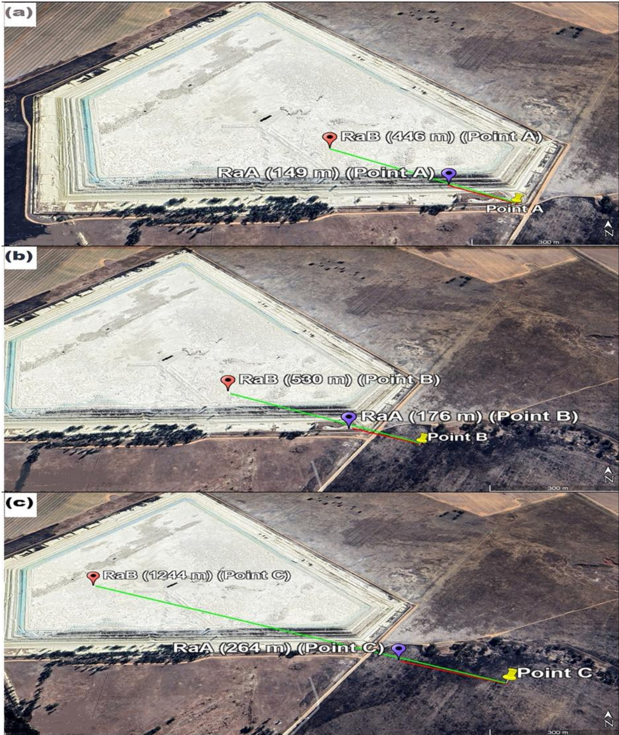
Figure 9: Day 3 afternoon radon source origins from back calculations for (a) receptor A, (b) receptors B and (c) receptor point C.
