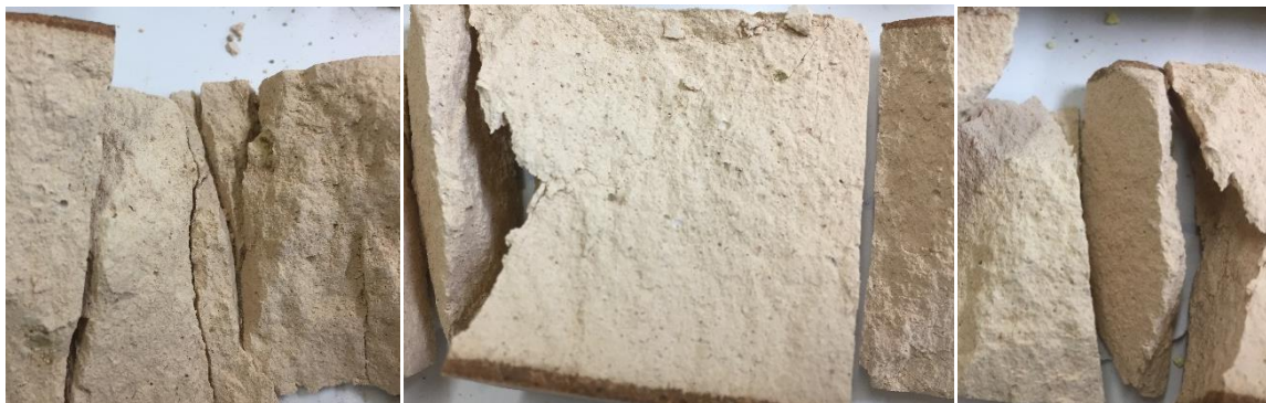
Figure 6: Aspects inside of monoliths (BNO in geopolimer matrix) after the compressive strength test.
