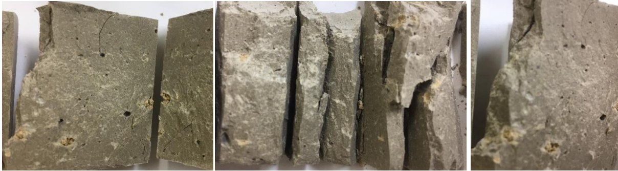
Figure 7: Aspects inside of monoliths (BNO in cement matrix) after the compressive strength test.
