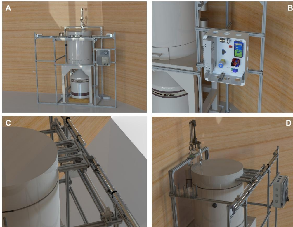
Figure 7: (A) Isometric view of the CAD design of the autosampler and its surroundings. (B) Detailed view of the CAD design of the interior of the electrical panel. (C) Detailed view of the CAD design of the door control subsystem. (D) Isometric view of the CAD design of both subsystems and the sample container rack.
