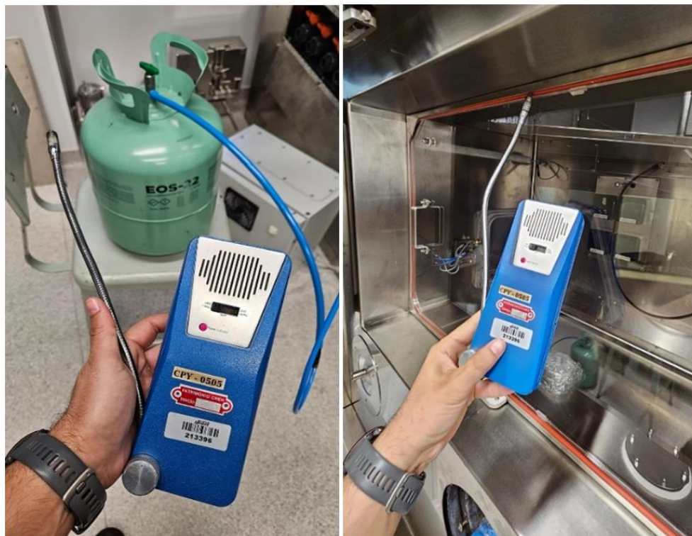
Figure 4: Leak detection with refrigerant R22.
