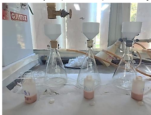
Figure 4: Filtrate collected for XRF analysis (Thermo QUANT ® X spectrometer) to quantify cesium
