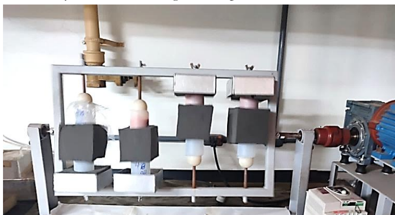
Figure 3: Rotary shaker according to the specifications of EPA Method 530
