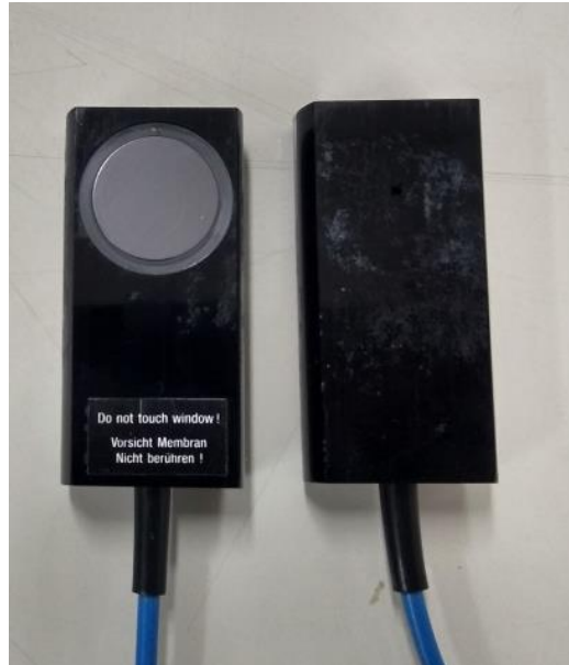
Figure 1: PTW brand parallel plate ionization chambers, model 23344.
