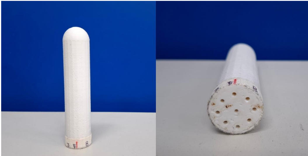
Figura 3: Cylindrical multi-channel applicator printed in PLA using a Raise3D Pro 2 Plus printer.
