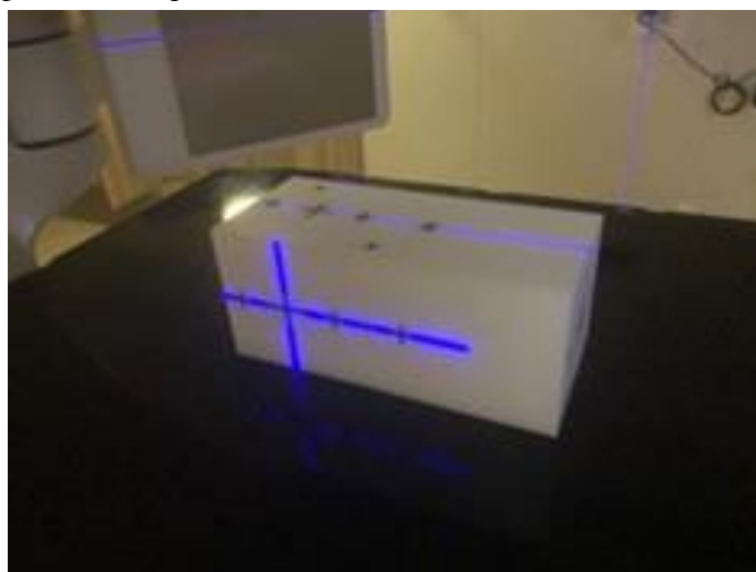
Figure 3: Setup for the acquisition of the Winston-Lutz test with the MultiMet-WL®
