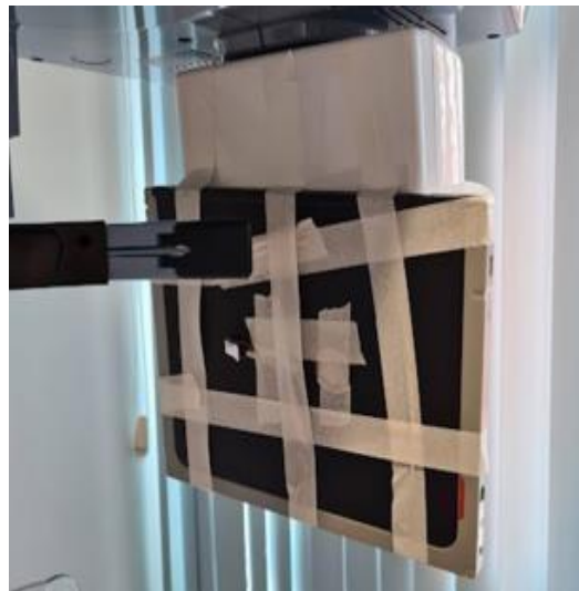
Figure 4: IP positioned on the image receptor to determine the field size used on irradiation
