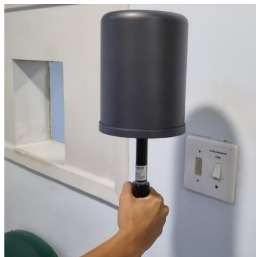
Figure 5: Ionization chamber positioned to perform the radiometric survey
