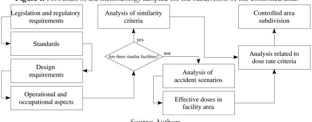
Figure 1: Flowchart of the methodology adopted for the subdivision of the controlled area.
