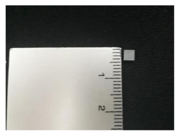
Figure 2: Thermoluminescent dosimeter.
